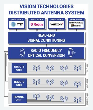
Optimizing patented technology for the transport of RF signals over fiber optics, our solutions utilize a broadband hybrid fiber/coax infrastructure to distribute voice and data services to mobile users throughout a building or campus. Radio Frequency (RF) signals from mobile networks are transported over the infrastructure to broadband antennas.
