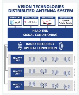
Optimizing patented technology for the transport of RF signals over fiber optics, our solutions utilize a broadband hybrid fiber/coax infrastructure to distribute voice and data services to mobile users throughout a building or campus. Radio Frequency (RF) signals from mobile networks are transported over the infrastructure to broadband antennas.
